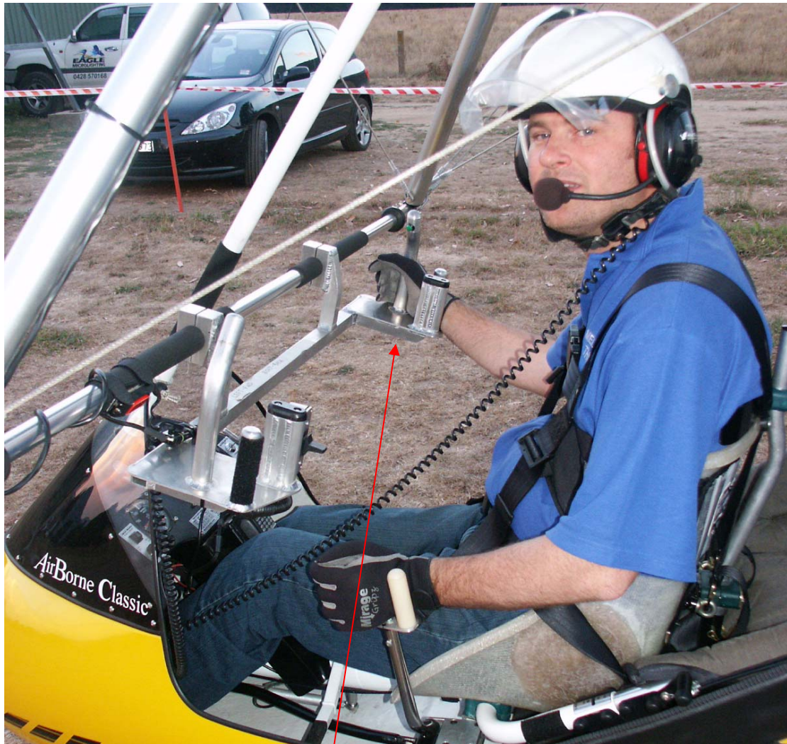
Control Bar with hand in position
