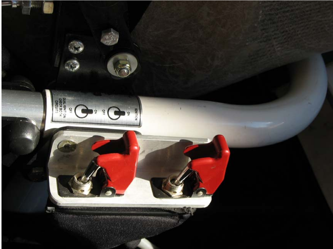
Figure 15 – On/Off Switches (shown in OFF position)
