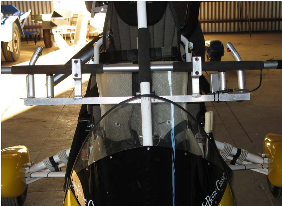
Figure 9 – Control Bar Clamped to Base Bar
