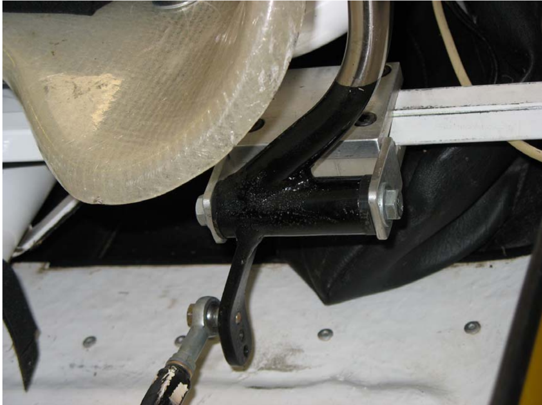
Figure 3 – Hand Steering Lever and Clamp Arrangement
