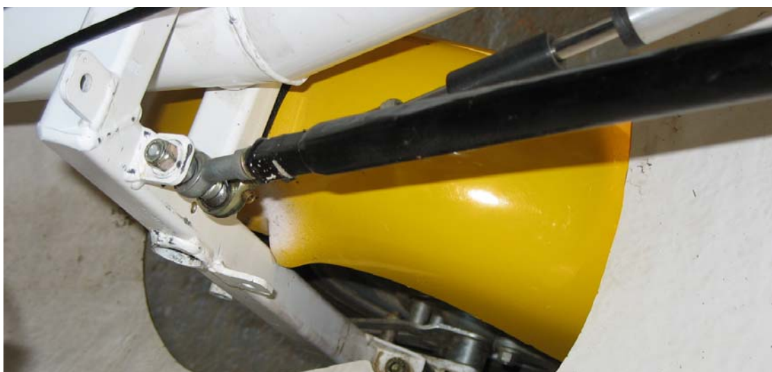
Figure 4 – Steering Rod & Fork Connection Point
