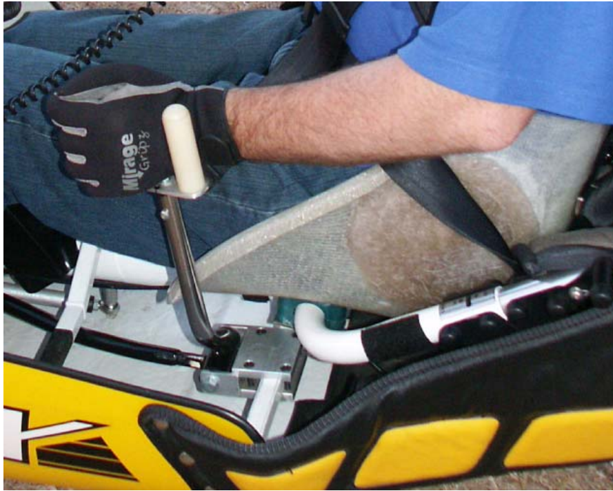
Figure 1 – Hand Steering Lever for Front Nose Wheel
